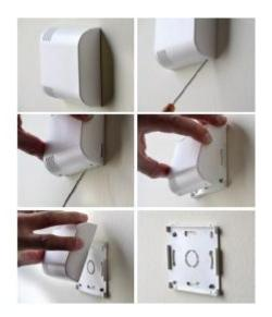
The sensor must be placed on the vertical inner wall (screws + bushings supplied), away from windows, direct sunlight, cold inlets or air vents and not above a radiator or any hot spot so as not to be subjected to excessively fast changes in temperature that may be detrimental to the quality of the measurements.
