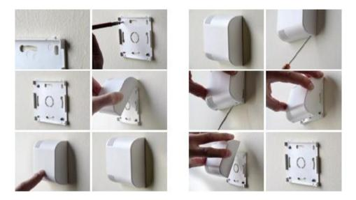
The sensor must be placed on the vertical inner wall (screws + bushings supplied), away from windows, direct sunlight, cold inlets or air vents and not above a radiator or any hot spot so as not to be subjected to excessively fast changes in temperature that may be detrimental to the quality of the measurements.
